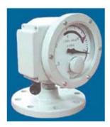
This level gauge detects the liquid title with the float, changes the measurement stroke into the turning angle degree through the tape for transmission, and directs the liquid title. The wireless pressure point of contact is supplied by using the cogwheel, the micro Switch, and the cam. Moreover, using the DC4-20mA output together is also possible according to the combination of the potentiometer and the R/I conversion machine.
