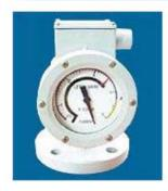
This level gauge is a small, cheap product. The structure detects the liquid title with the float, changes the measurement stroke into the turning angle degree through the tape for transmission, and directs the liquid title. The wireless pressure point of contact is supplied by using the cogwheel, the Micro Switch, and the cam.
