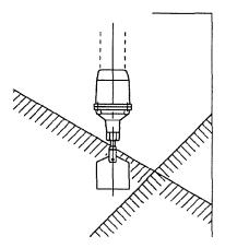
b. Impact of powder and particles When the level switch is mounted just under the point where powder and particles fall, it may be broken by impact such as an arching phenomenon in the hopper. Change the mounting location or mount a protection plate.
