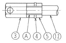
The screw (A) is a left-handed type. The nut (5) is screwed on the shaft (12) to put the spring washer in and the paddle boss (3) is screwed on. Keep in mind that a screw lock agent is used for the screw portion.
