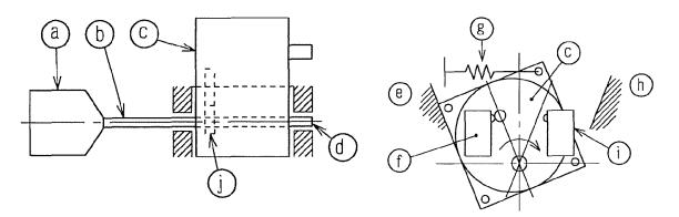
The motor (c) is placed at a position (e) because of the spring (g) and the shaft (b) rotates with the mounted paddle (a). If rotation of the shaft (b) is restricted by sediment together with the paddle (a), the motor (c) overcomes the spring (g) by the internal reduction gear (j) to rotate around the shaft of motor (d) and tilt toward the (h) side, and the level detection signal is output by the micro switch (f). Then, the motor (c) is stopped by the micro switch (i).
